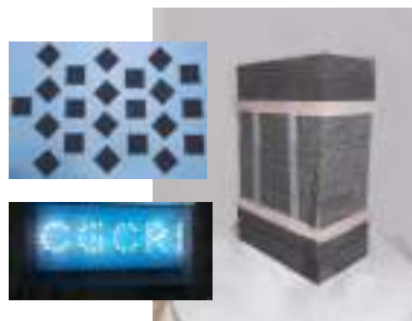
500W Class Working SOFC Stack (Inset: SOFC single cells & illumination by SOFC power)
